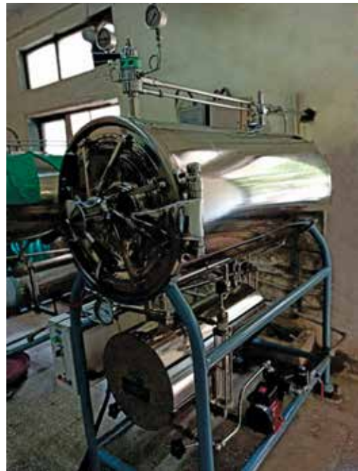
Horizontal Cylindrical High Pressure Steam Sterilizer donated to Cama & Albless Hospitals Mumbai
